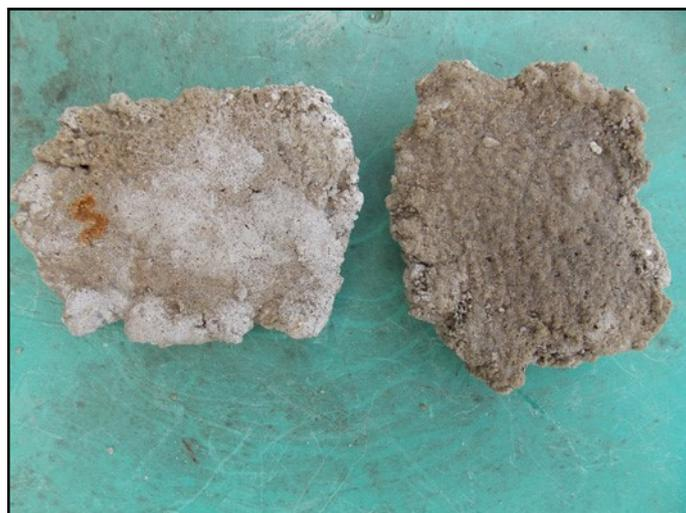
The two pieces were left in a dry garage and checked periodically. After a few months they appeared to be completely dry and quite hard, though it was possible to snap off small pieces by hand. At this stage it was considerably firmer than lime mortar but not as firm as cement. It was left in the garage, and continued to harden. Although one piece contained salt and the other did not, they both appeared identical.
